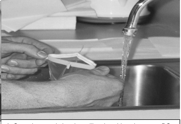
2. Open the sample bag by pulling the white tabs apart. DO NOT TOUCH THE INSIDE OF THE BAG.
